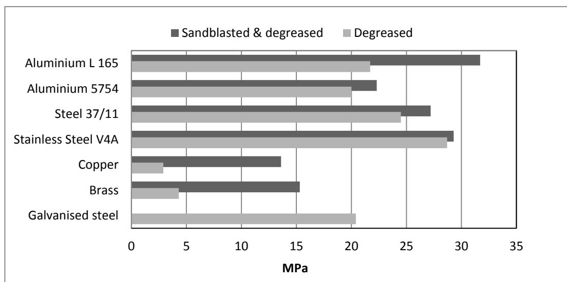
Notes: Araldite® 2051 is not suitable to bond copper or brass without surface preparation. Galvanised steel should not be abraded or sandblasted, better results are obtained with only degreasing.
