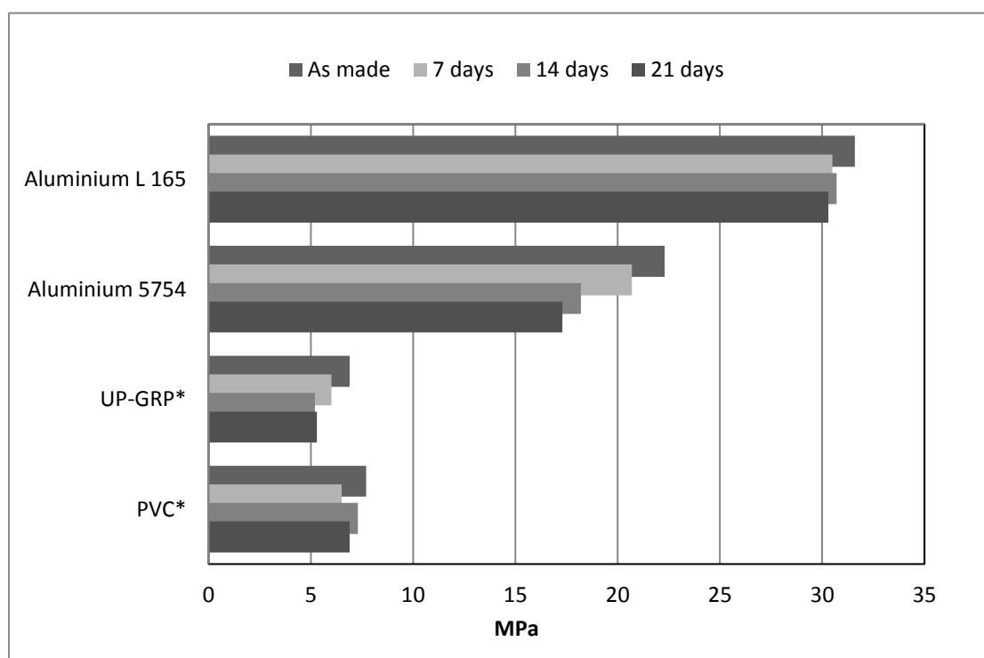
(\*): UP-GRP, PVC, substrate failure
